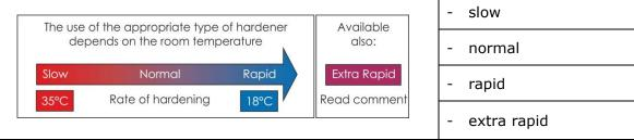
The type of used hardener affects coating drying time and depends on room temperature and the preference of the painter. Proper selection of the type of hardener ensures appropriate structure and appearance of coating.
